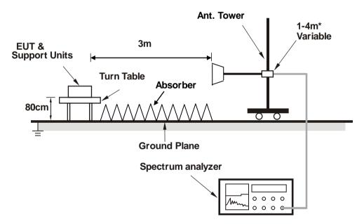
\*:depends on the EUT height and the antenna 3dB beamwidth both.
